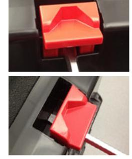
To remove a damaged locker system, flip tote over on the side and approach tote from the bottom of base. Insert a large flat blade screwdriver in middle of locking carriage as shown. Lightly pry carriage upward out of base opening. Remove and discard old locking carriage.
