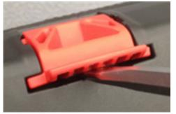
To remove a damaged locker system, flip tote upside down and approach tote from the bottom of base. Insert a large flat blade screwdriver in middle of locking carriage as shown. Lightly pry carriage upward out of base opening. Remove and discard old locking carriage and spring.
