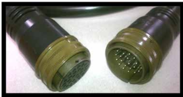
Figure 6. Cable with aluminum cable coupler ring.
