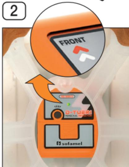
Fasten the Dual Lock tape provided with the detector to the centre of the helmet, as shown in the picture, and press down hard for approximately 20 seconds.
