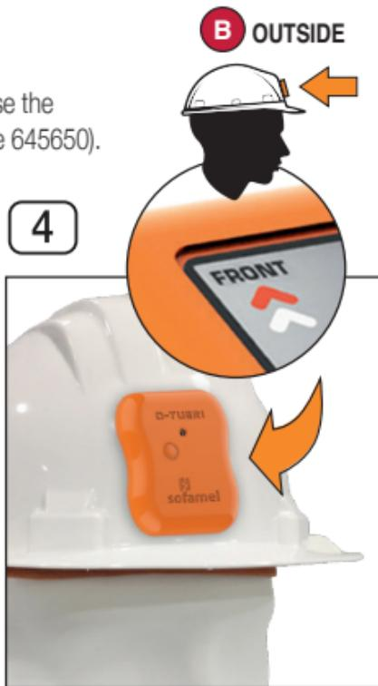
Fasten the Dual Lock tape provided with the detector to the centre of the helmet, as shown in the picture, and press down hard for approximately 20 seconds.
