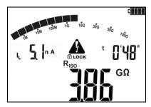
Use **SET/SEL** to display values of leakage current  $I_L$ .
