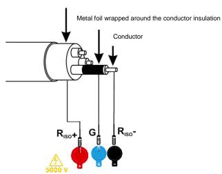
The same shall apply when measuring the resistance between two conductors of the cable, attaching to **G** terminal other conductors that do not take part in the measurement.
