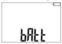
The battery pack is fully discharged,
