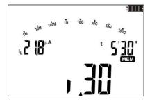
The value of leakage current I<sub>L</sub> measured in time t=5'30'. Symbol J I indicates the selected time interval, in which the leakage current value was recorded.
