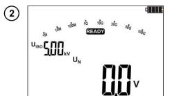
The meter indicates readiness for measurement with increasing voltage.
