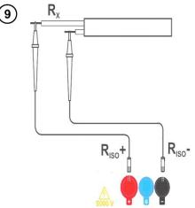
Connect test leads according to the drawing.
