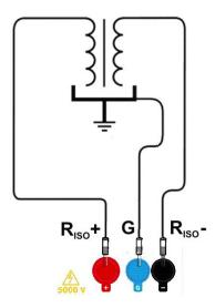
when measuring insulation resistance between one of the cable conductors and the cable jacket, the effect of surface resistances (important in difficult weather conditions) is eliminated by connecting a piece of metal foil insulating the tested conductor with G socket of the meter;
