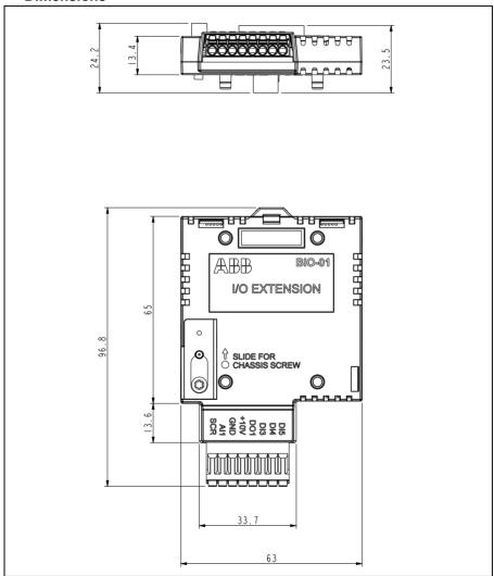
Note! BIO-01 is supplied with a high cover part (part no 3AXD50000190188) that increases the drive depth by 15 mm (0.6 in).
