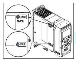
screw in the EMC filter location. To connect the filter, remove the plastic screw and insert the metal screw and washer from the hardware bag shipped with the drive.
