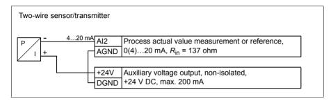
Note: The sensor is supplied through its current output and the drive feeds the supply voltage (+24 V). The output signal must be 4...20 mA, not 0...20 mA.
