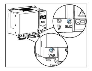
WARNING! If you connect the drive to an IT system (an ungrounded power system or a high-resistance-grounded [over 30 ohms] power system), disconnect the varistor from ground. Failure to do so can cause damage to the varistor circuit.
