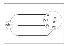
Moisture in the motor casing decreases the insulation resistance. If you think that there is moisture in the motor, dry the motor and measure again.
