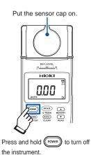
6 When the measurement is finished, put the sensor cap on and turn off the instrument.
