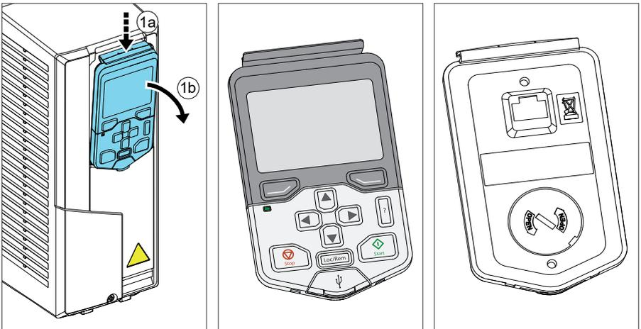
To reinstall the control panel, put the bottom of the container in position (1a), press the retaining clip at the top (1b) and push the control panel in at the top edge (1c).
