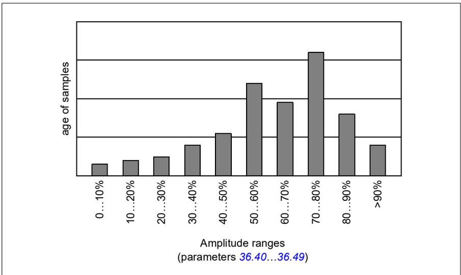
Amplitude logger 1 is fixed to monitor motor current, and cannot be reset. With amplitude logger 1, 100% corresponds to the maximum output current of the drive ( $I_{\max}$ ), which is listed in the *Hardware manual* of the drive. The measured current is logged continuously. The distribution of samples is shown by parameters [36.20](#)...[36.29](#).
