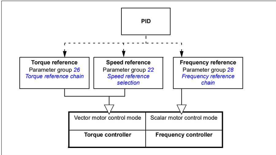
The following is a more detailed representation of the reference types and control chains. The page numbers refer to detailed diagrams in chapter [Control chain diagrams](#).
