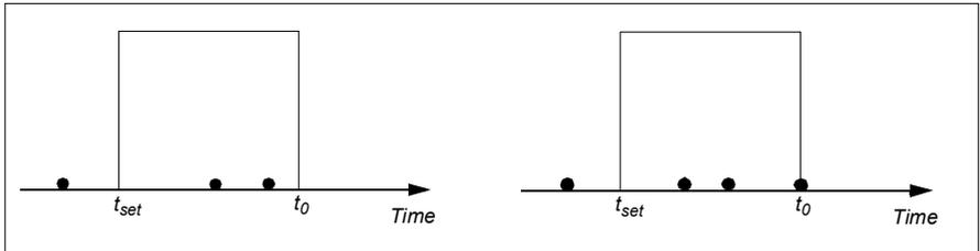
The third pump cleaning cycle starts within the preset count time (one hour) and the pump cleaning function trips on a fault and the pump is stopped without performing the third cleaning cycle. After resetting fault, the drive starts with the third pump cleaning cycle.
