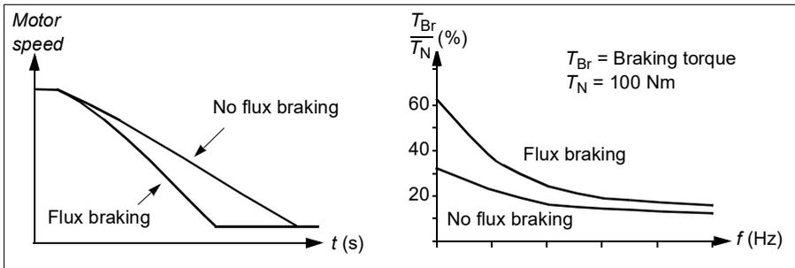
The drive monitors the motor status continuously, also during flux braking. Therefore, flux braking can be used both for stopping the motor and for changing the speed. The other benefits of flux braking are:
