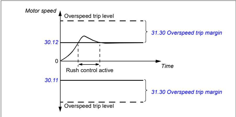
The function is based on a PI controller. The proportional gain and integration time can be defined by parameters. Setting these to zero disables rush control.
