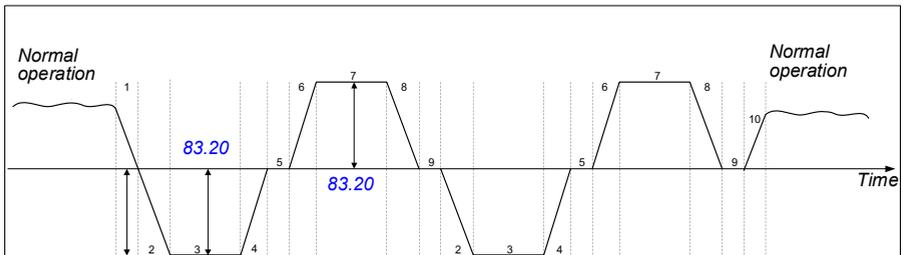
The time from zero speed to [83.20 Cleaning speed step](#) is considered as Time to zero speed.
