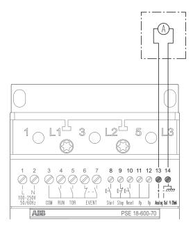
Figure 5.15: Terminals for analog output
