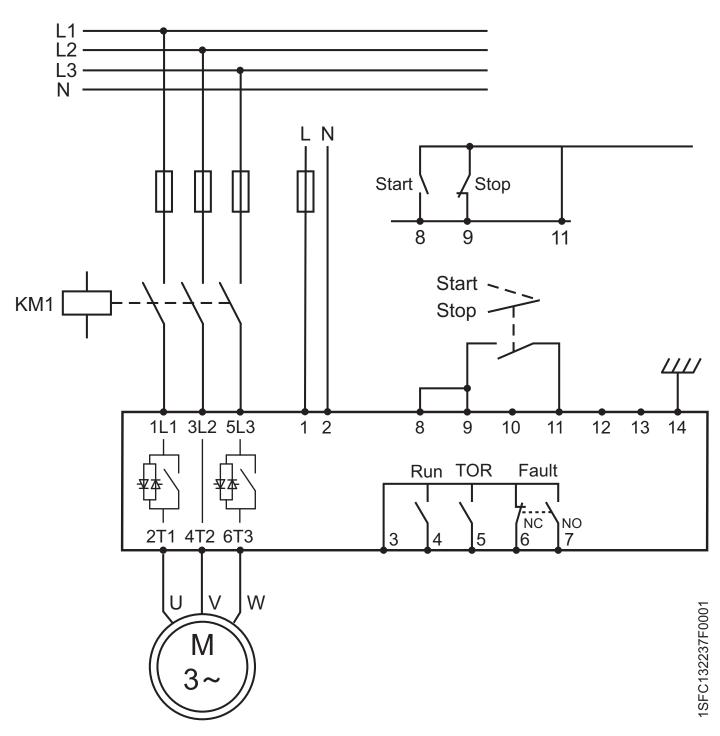
Circuit diagram PSE18...PSE370 (Fuse and contactor version)
