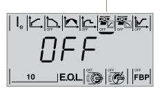
Figure 7.14: Torque Control during start ramp parameter displayed
