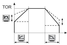
Figure 7.9: The function of Initial/End Voltage
