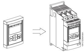
Figure 5.22: Transfer of parameters from external keypad to softstarter
