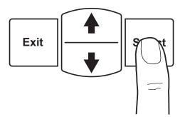
Figure 6.6: Enter Settings Level pressing the Select key.
