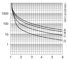
Figure 7.21: Tripping curves for the Electronic Motor Overload Protection (E.O.L.)
