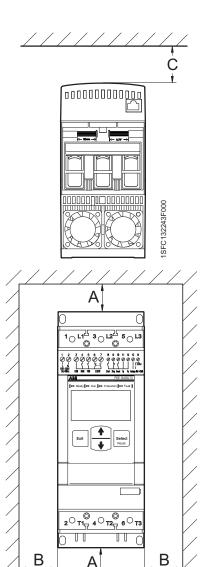
Figure 4.5: Minimum distances to wall and front
