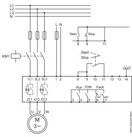
Figure 5.1: Connection of PSE Softstarter and connection in series with a line contactor.
