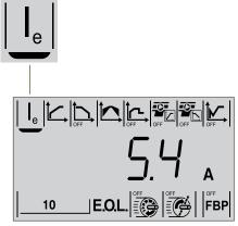
Figure 7.3: Rated Current parameter displayed
