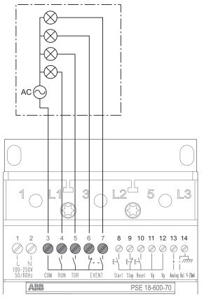
Figure 5.17: Terminals for status output signals
