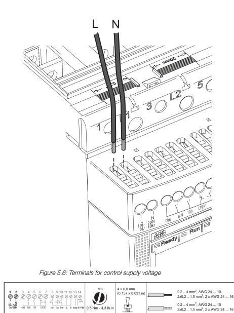
Figure 5.7: Tightening torques and wire area
