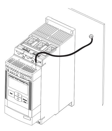
Figure 5.8: Terminal for functional earth
