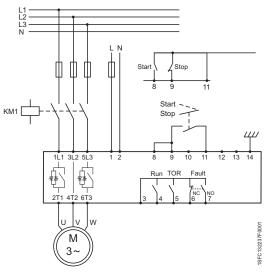
Figure 2.2: Example connection of PSE Softstarter
