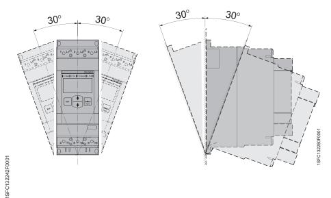
Figure 4.6: Maximum mounting angle
