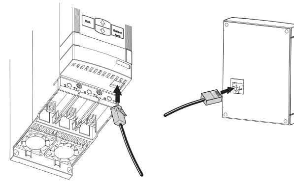
Figure 5.20: Connection of external keypad
