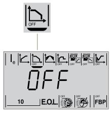
Figure 7.6: Stop Ramp Time parameter displayed
