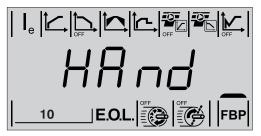
Figure 7.31: Type of operation for reset of Fieldbus fault parameter displayed
