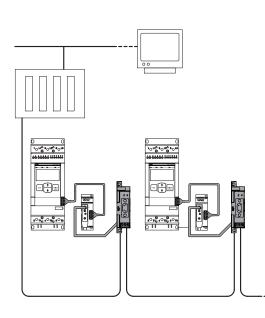
Figure 8.1: Principle of a fieldbus network with PSE Softstarters connected
