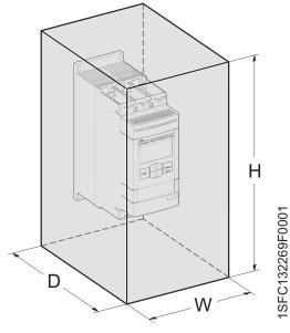
Figure 4.3: Dimensions minimum enclosure size
