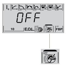
Figure 7.25: Locked Rotor Protection parameter displayed
