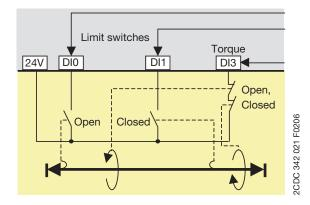
DIO: Motor off, start only in Closed direction
