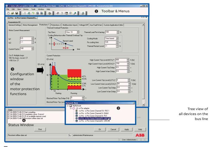
UMC100.3 configuration tool Asset Vision Basic with the motor protection configuration window ②. In ① the toolbar of the tool is shown. ② provides a network view with all the devices accessible on the PROFIBUS DP line. ② contains a window to display messages and buttons to quit or adopt the parameter changes.
