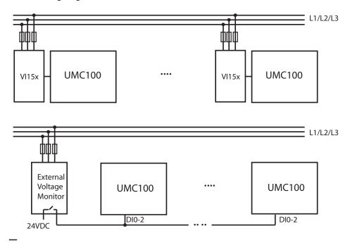
A low voltage situation can be detected either by the VI15x module or using an external voltage monitoring relay. In the latter case the low voltage signal has to be wired to all motor controllers
