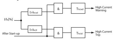
Signal flow of the high current protection function.
