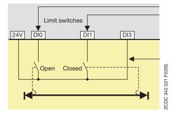
DIO: Motor off, start only in Close direction DI1: Motor off, start only in Open direction
