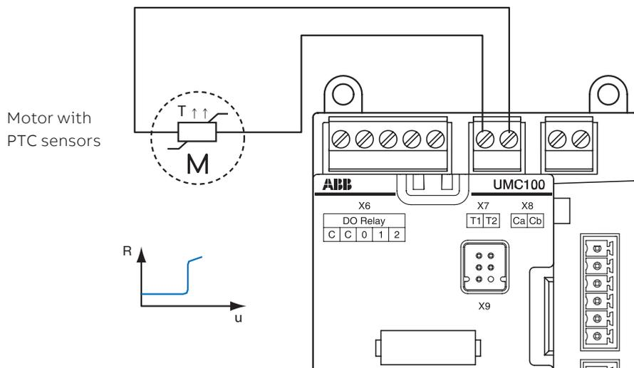
**Connect the PTC to the T1/T2 terminals of the UMC**
