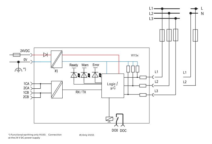
Wiring diagram of the VI15x modules
