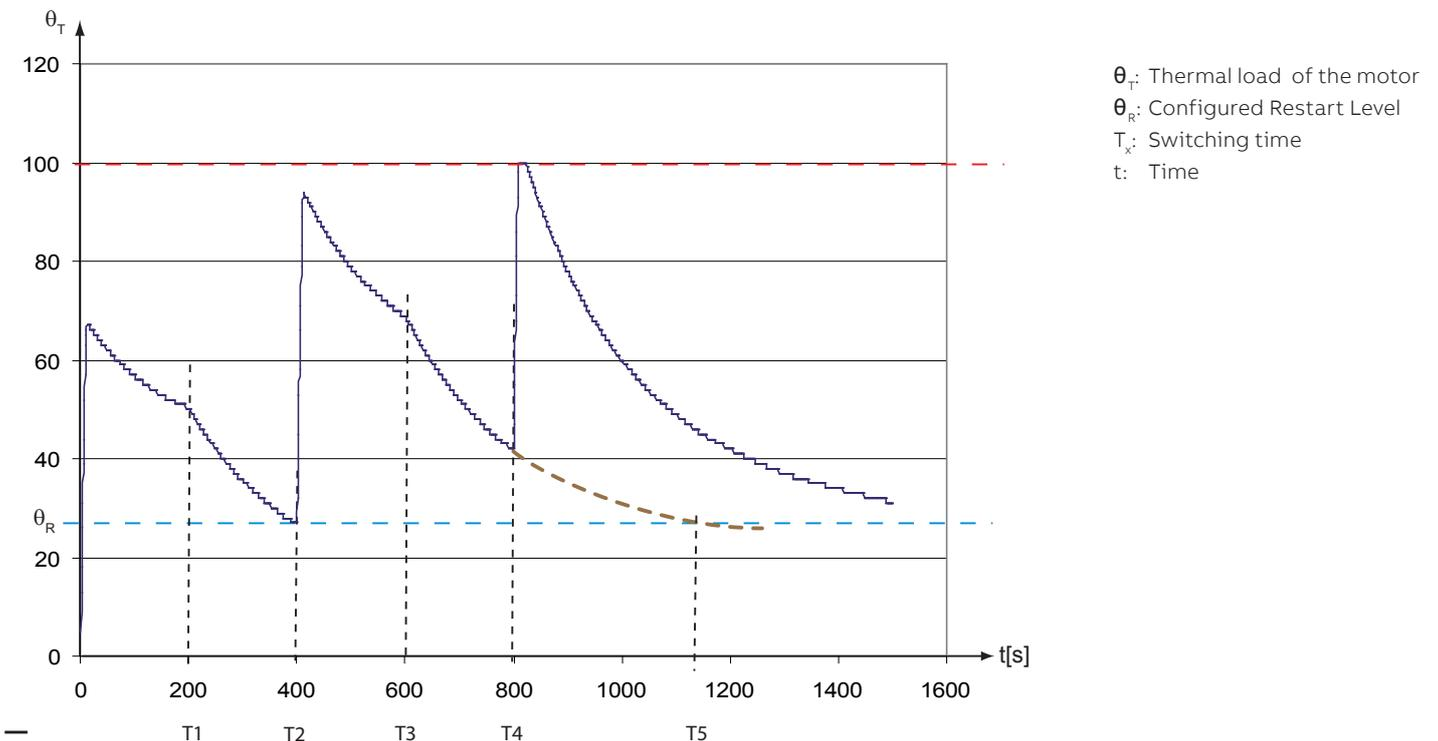
**Trend of the calculated motor temperature after several starts.**
