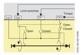
DIO: Preparation for Open limit motor off
