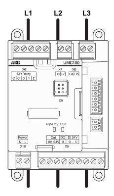
If the phase sequence supervision is active the phases must be fed through the UMC in the shown order
