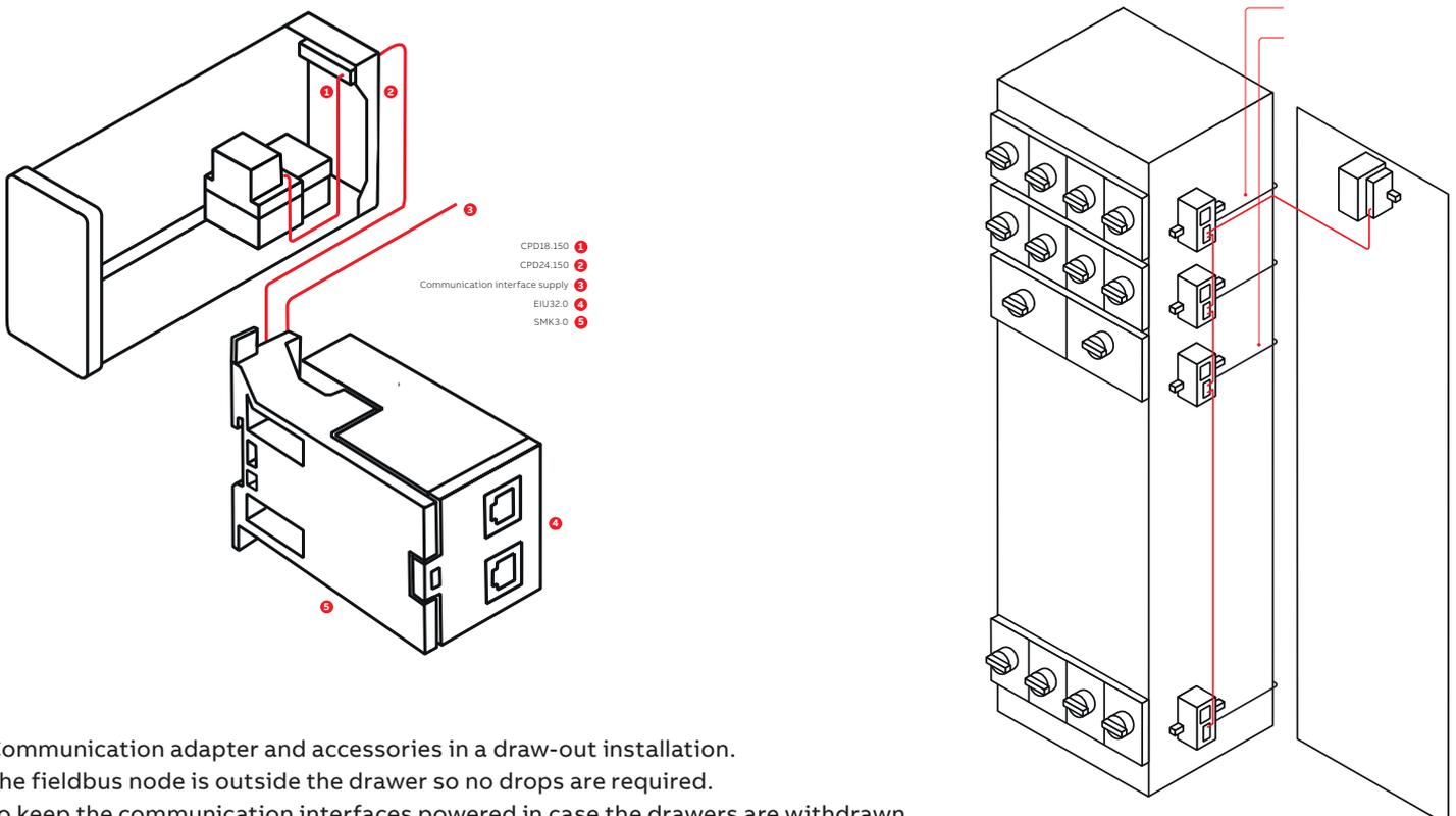
Communication adapter and accessories in a draw-out installation. The fieldbus node is outside the drawer so no drops are required. To keep the communication interfaces powered in case the drawers are withdrawn they must be powered separately (not shown here).
