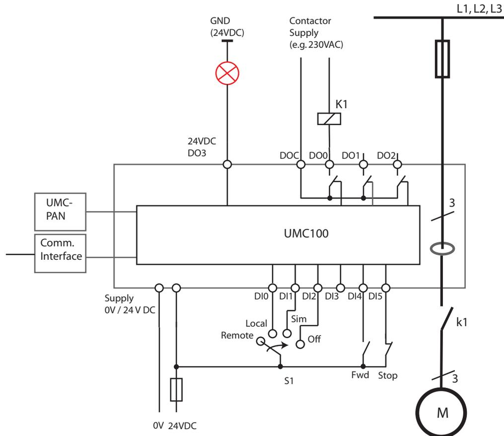
From the requirements you can see that the three control places Digital Inputs, Fieldbus and LCD are used.
