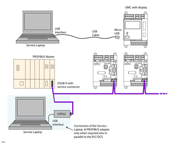
Connection of a service laptop using a USB cable connected with the UMC100 LCD panel (point-to-point) or UTP22-FBP (for a whole PROFIBUS line)
