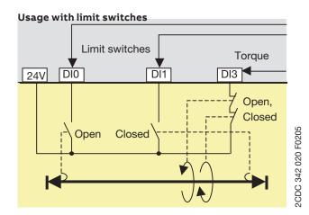
DIO: Motor off, start only in Closed direction DI1: Motor off, start only in Open direction
