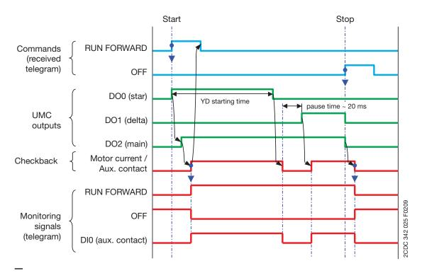
Timing Diagram for Star-Delta Starter
