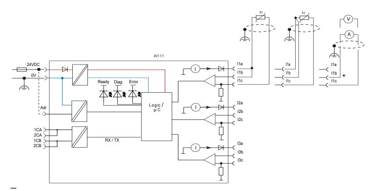
Wiring diagram of the Al111 modules. Depending on the analog input source choose the correct terminals
