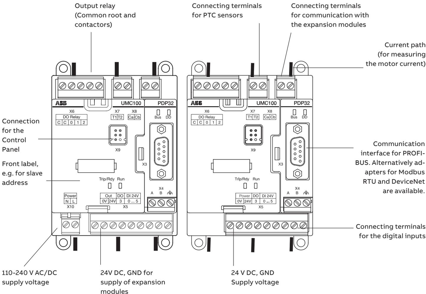
After powering on, the UMC100.3 performs a self-test of its hardware and checks the configuration for consistency. In the event of a failure, a self-test fault is generated and signalled. Replace the device in such a case. After a successful self-test the UMC enters the operational state.
