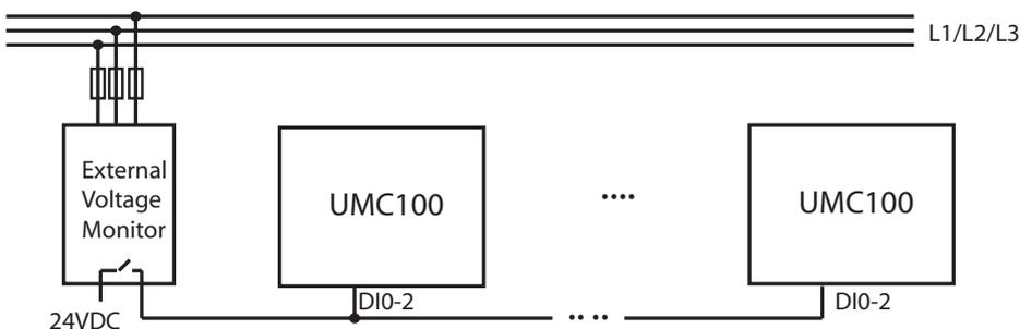
**A low voltage situation can be detected either by the VI15x module or using an external voltage monitoring relay. In the latter case the low voltage signal has to be wired to all motor controllers**
