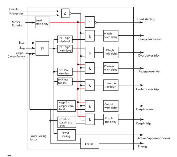
Block diagram showing the data flow of the power protection function. The signals on the right are available for further processing e.g. in a user defined custom application
