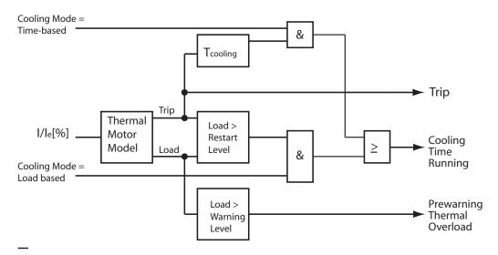
Signal flow of the thermal overload protection
