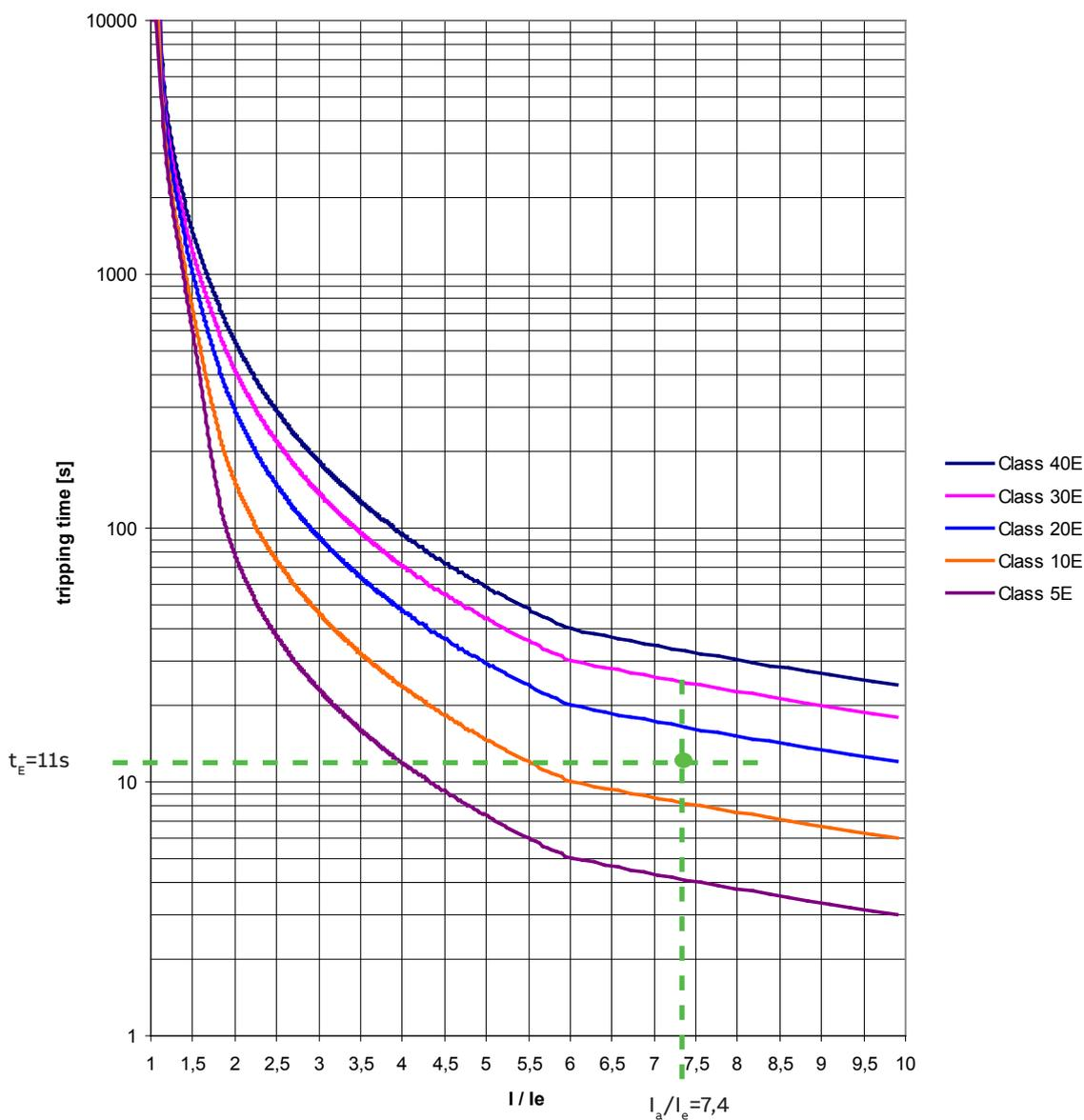
**Example for the trip class selection for a given motor**
