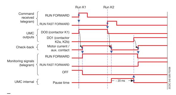
**Timing Diagram for Pole-Changing Starter**
