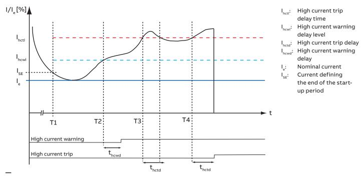
Trend diagram of the motor current over time
