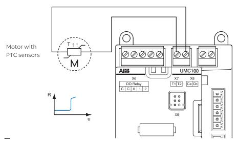
Connect the PTC to the T1/T2 terminals of the UMC
