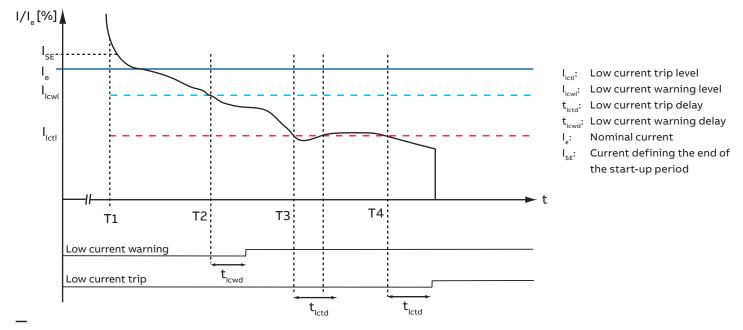
Trend diagram of the motor current over time
