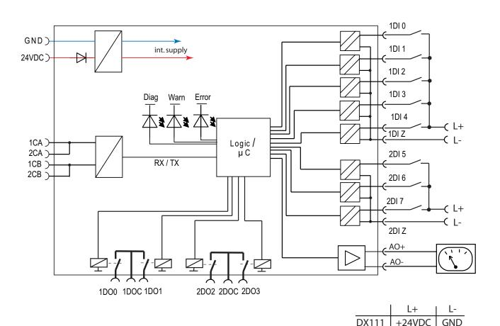
Wiring diagram of the DX111-FBP.0 and DX122-FBP.0 module
