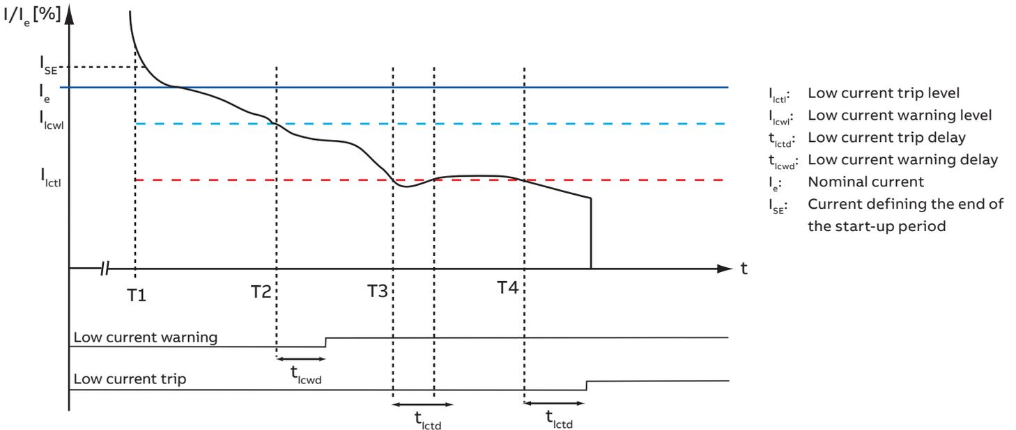
**Trend diagram of the motor current over time**
