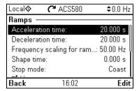
Use the Ramps submenu to set up acceleration and deceleration settings.
