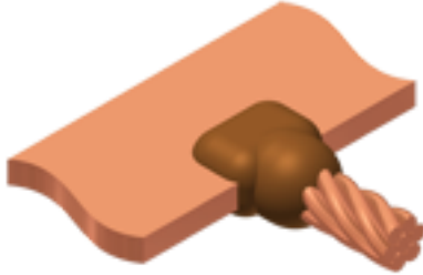
Horizontal Cable Horizontal Bus Bar
