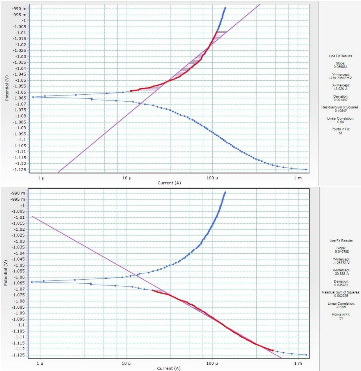
Figure 7: Potentiodynamic polarization curve, line fit results for the anodic Tafel and cathodic Tafel regions of Test 1 for a galvanized steel rod embedded in Conducrete for 21 days
