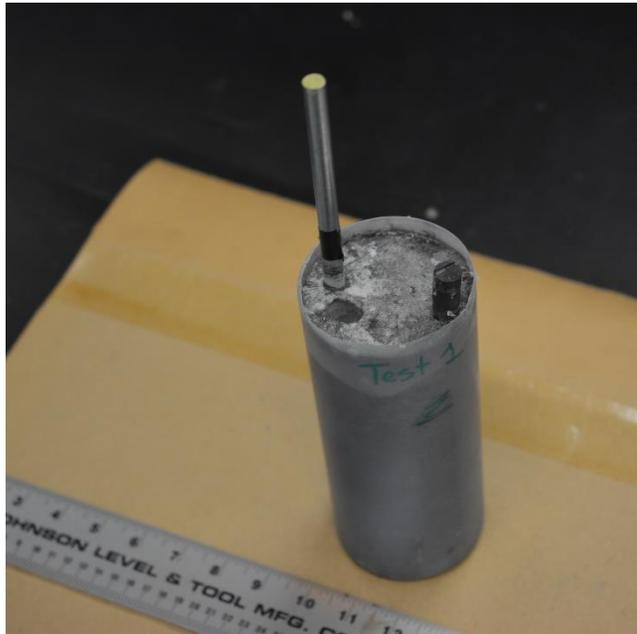
Figure 1: Image of the sample for LPR tests of galvanized steel embedded in Conducrete
