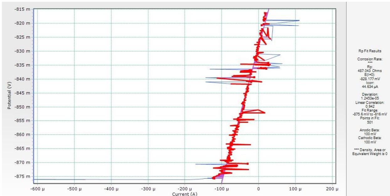
Figure 3: Linear polarization curve and the polarization resistance (Rp) fits for Test 2 for a galvanized steel rod embedded in Conducrete for 21 days-LPR tests were conducted at room temperature
