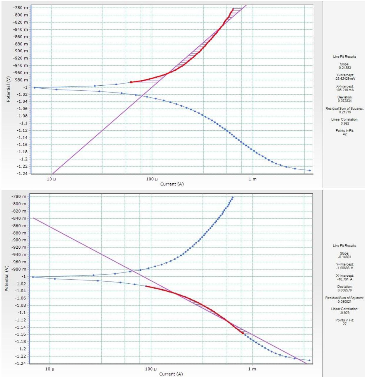
Figure 6: Potentiodynamic polarization curve, line fit results for the anodic Tafel and cathodic Tafel regions of Test 1 for a galvanized steel rod embedded in Conducrete for 21 days
