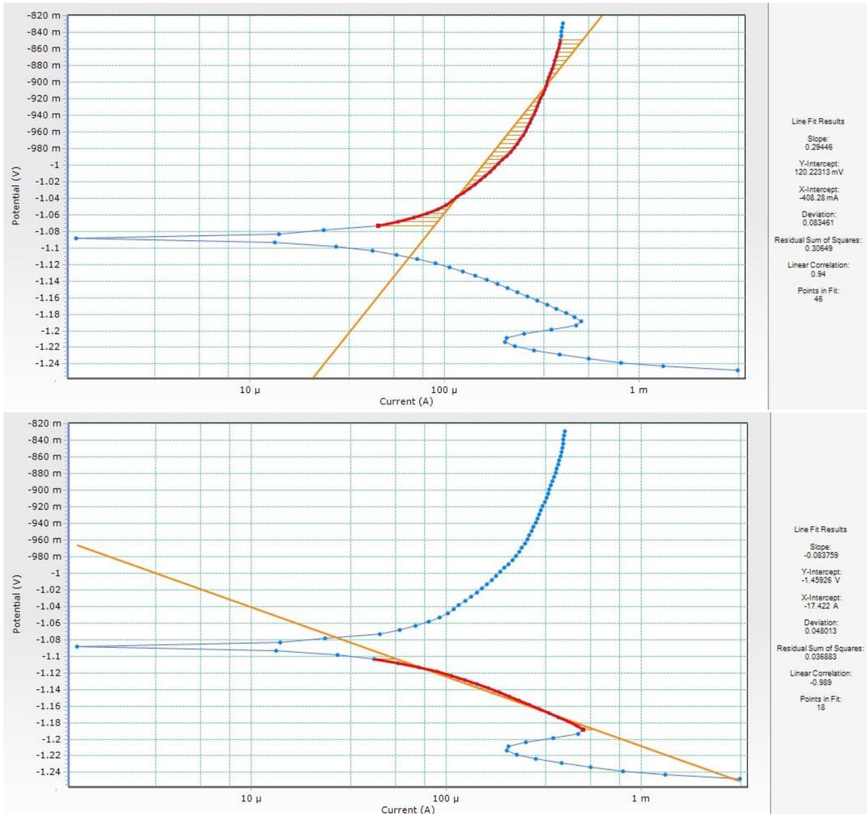
Figure 5: Potentiodynamic polarization curve, line fit results for the anodic Tafel and cathodic Tafel regions of Test 1 for a galvanized steel rod embedded in Conducrete for 21 days
