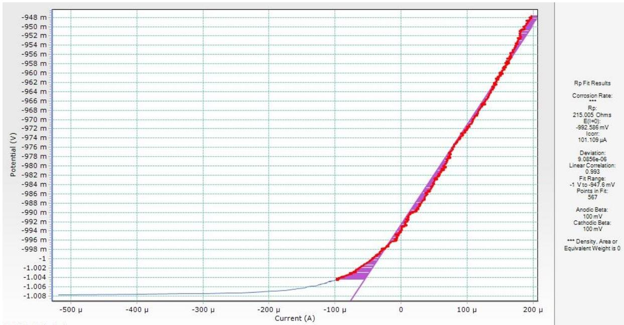
Figure 4: Linear polarization curve and the polarization resistance (Rp) fits for Test 3 for a galvanized steel rod embedded in Conducrete for 21 days-LPR tests were conducted at room temperature
