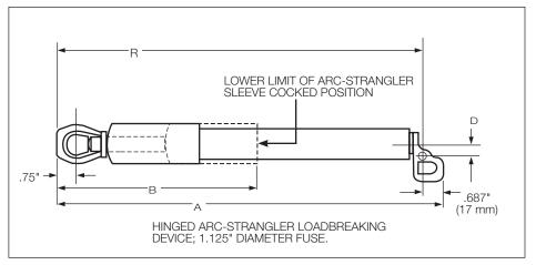
Figure 7. NX hinge-style (1.125" dia.) fuse dimensional drawing.
