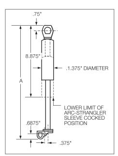
NX hinge-style switchblade with Arc-Strangler loadbreaking device. (See Table 5 for dimensions.)
