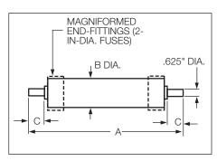
Figure 5. NX clip style dimensional drawing. (See Table 4 for dimensions.)
