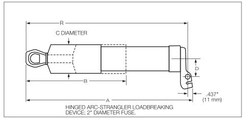
NX hinge-style (2" dia.) fuse dimensional drawing.
