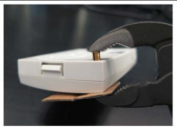
3. Cover the front of the panel and squeeze the insert into the panel with pliers.
