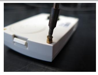
3. Heat the soldering iron to 350°C and heat the insert for two seconds.
