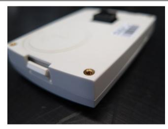
4. Make sure the insert is in level with the panel's back cover
