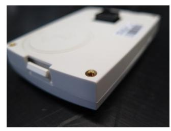
4. Push the insert into the hole with the hot soldering iron. Make sure the insert is in level with the panel's back cover
