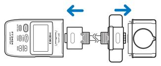
Do not seperate and connect the display unit and the sensor unit while the instrument power is on.
