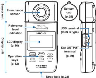
Lux meter could be seperated into sensor unit and display unit. (p. 33) (Use the option L9820 Connection cable)
