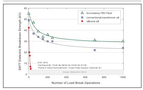
Figure 5. Fluid loadbreak dielectric strength retention comparison.
