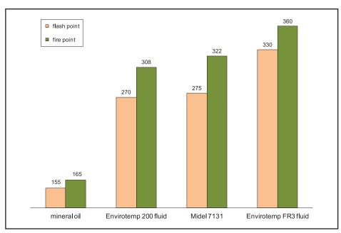
Figure 2. Flash & Fire Point of Dielectric Fluids (°C).
