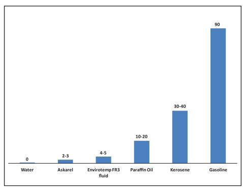
Figure 3. Fire Hazard Rating UL Standard 340.
