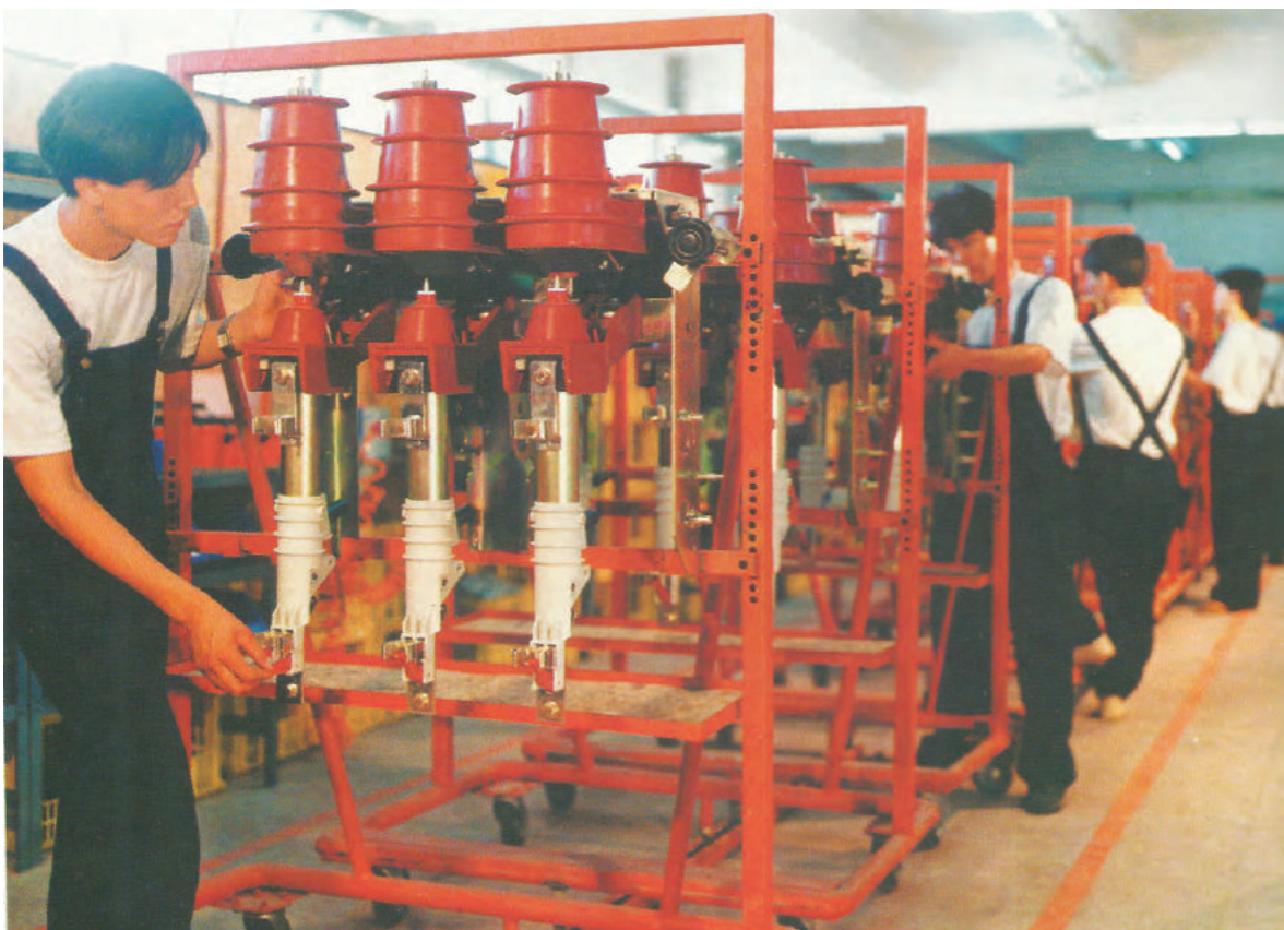
Load Break Switch assemble line in our factory
