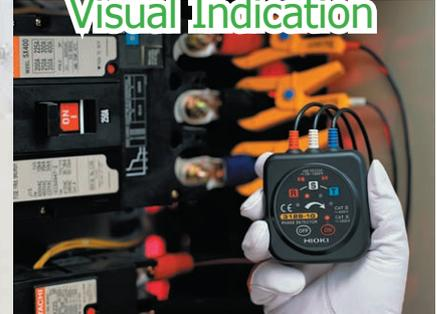
Based on the electrostatic induction theory, the 3129 series Phase Detectors can safely and accurately detect phase sequence in three-phase circuits. Correct sequence is indicated by a crystal clear beeping tune, while bright red LEDs show sequence direction.
