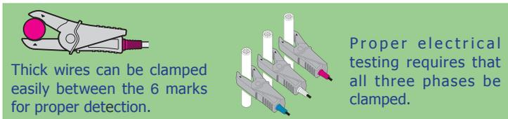
Thick wires can be clamped easily between the 6 marks for proper detection.
